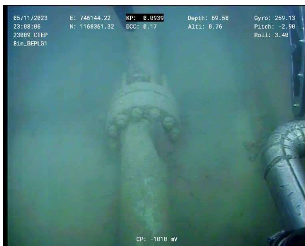
Figure 7 – BEWG Spool Tie-in Flange KP 0.094 (Top View)
