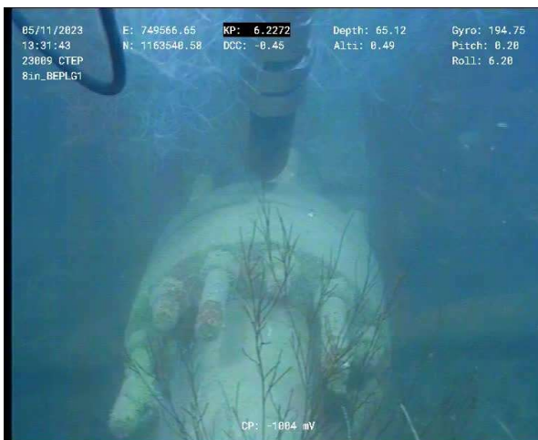
Figure 11 – BEWA Riser Tie-in Flange KP 6.227 (Top View)
