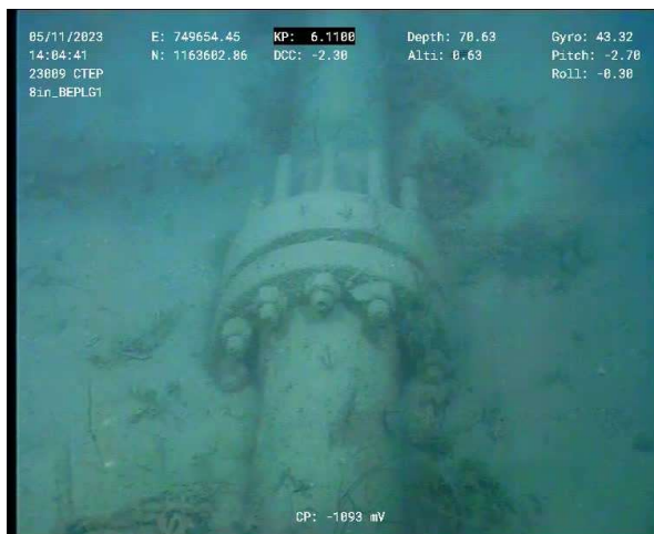
Figure 17 – BEWA Spool Tie-in Flange KP 6.110 (Top View)
