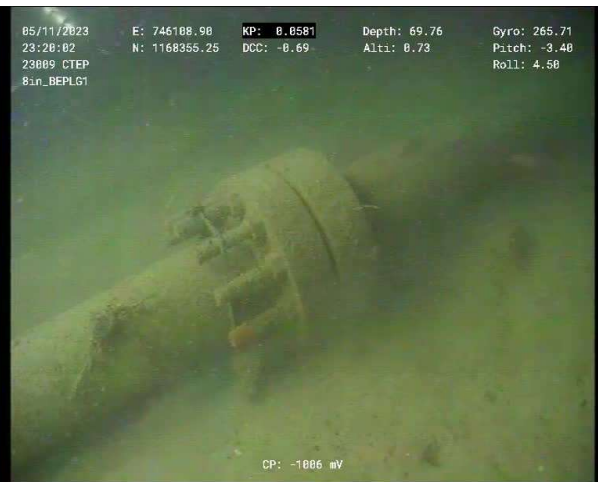
Figure 6 – BEWG Spool Tie-in Flange KP 0.057 (Side View)
